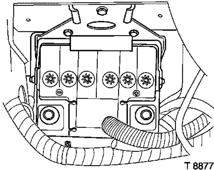
5. Remove battery clamp from bulkhead
